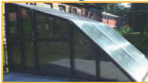
Head based storage Solar Kiln
