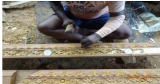
Then the sharp pointed chisel is used for sculpturing
