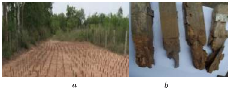
Fig. 2 (a) Samples exposed to open field conditions for assessing durability class, (b) Samples attacked by insects
