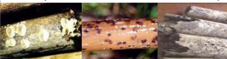
Fig. 1 Wood decay by fungus and insect
