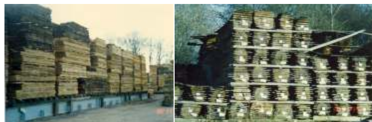
Fig. 3 Air drying of wood
