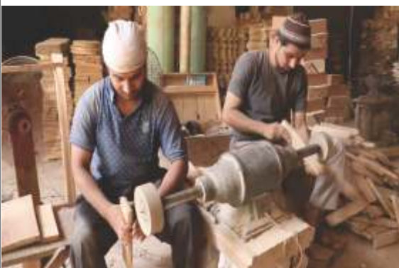
Wood grinding is manually done to make intricate shaped articles
