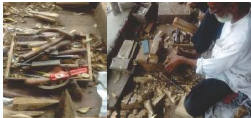
Wooden hammer, various types of chisels and scooping tools are used in carving
