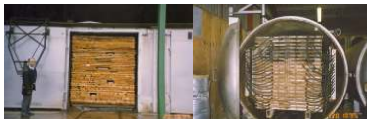
Steam heated kiln
